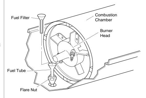
Figure 8 - Fuel Filter Removal, 150,000 BTU/Hr Model
